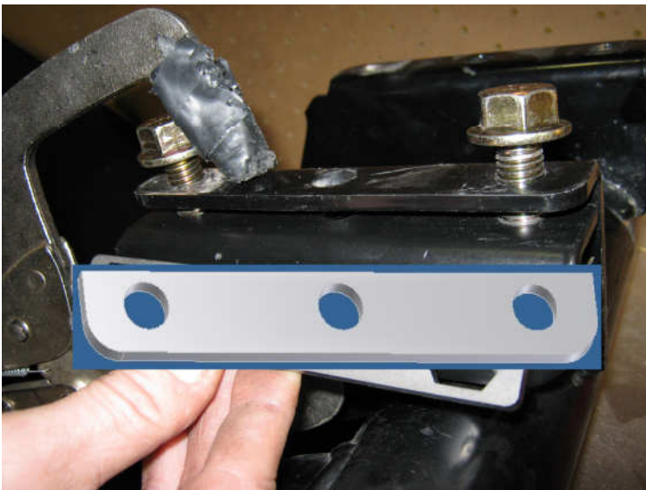
Figure 6. The shim plate fits between the trunion plate and the trunion mount.
