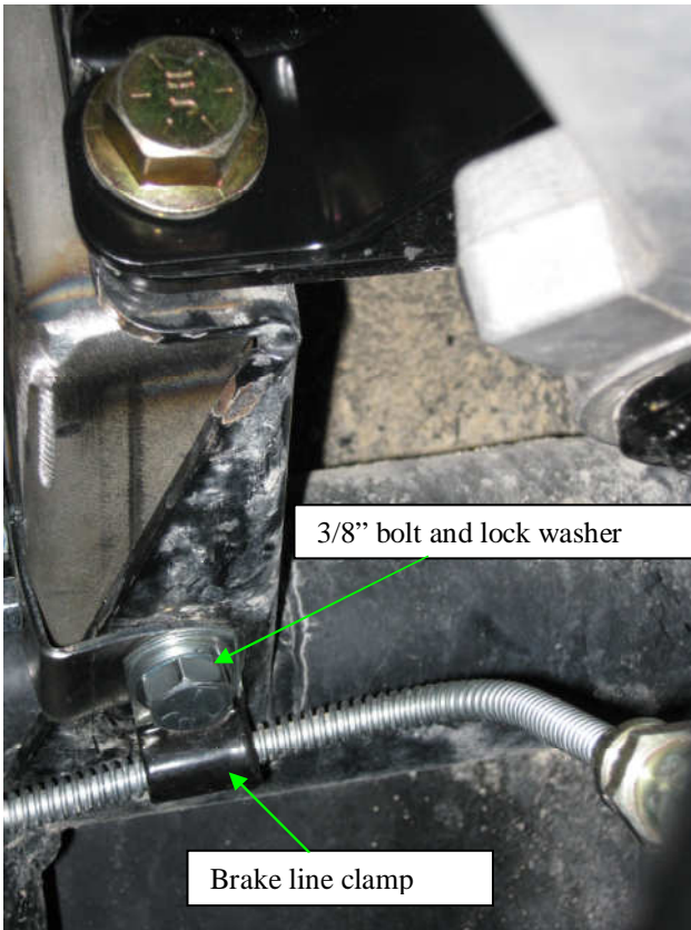
Figure 12 Brake line installations
